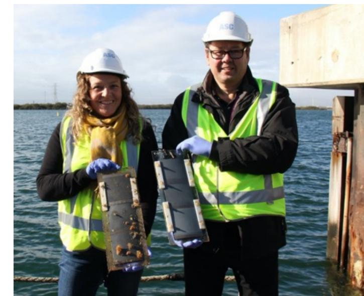
Figure 1. Biofilm formation on conducting coatings after 55 days in in Port River (April-June), Adelaide. Control coupon (left) and a coupon exposed to intermittent electrochemical stress (right) during the experiment.
