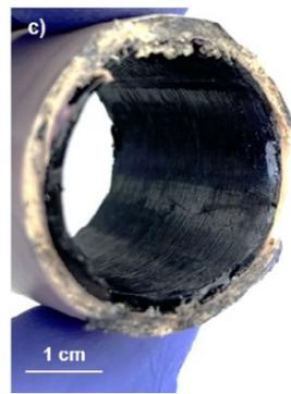
Figure 1A. a) Synthesis pathway of oligomer (1) and curing process to access cross-linked polymer. b) Polymer coated silica gel. c) Polymer coated, solvent resistant PVC pipe.
