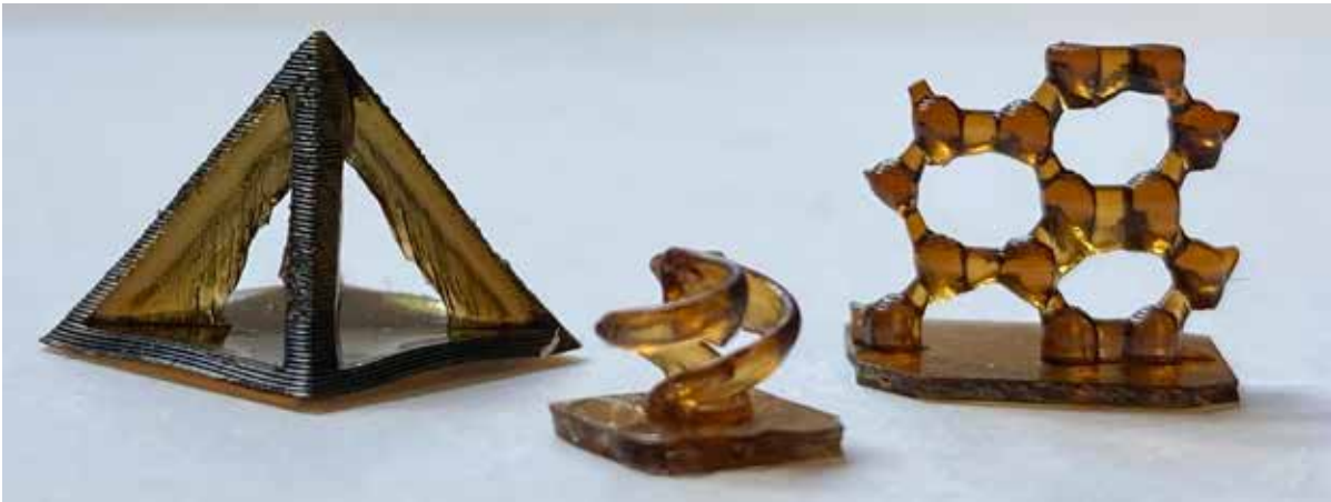
Figure 1 3D printed structures using dual-cure resins.
