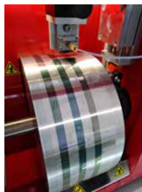
Figure 1 Mini-roll coater with slot-die attachment actual image of device (left) and schematic (right).
