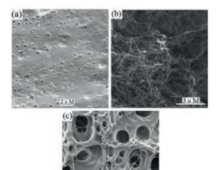
FIGURE 1 SEM images of (a) PAA, (b) BC, and (c) BC-PAA
