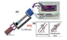
**CONTROLLING SELF-ASSEMBLY** The vortex fluidic device (VFD) is effective in controlling the self-assembly of materials, including fullerenes, into functional materials.
