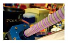
**ORGANIC SYNTHESIS & CATALYSIS** Attaching enzymes and catalysts in general to the surface of the VFD tube allows catalytic reactions at the different zones along the tube, under continuous flow – scalable processing.
