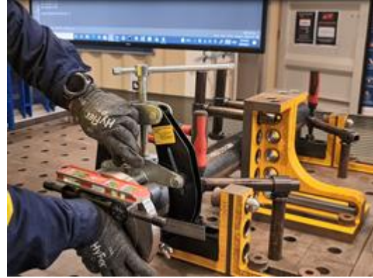
Figure 3.d: Manoeuvring the wing nuts allows adjustment of the flange position and orientation to the clamped pipe.
