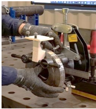
Figure 4.a: Performing flange-to-pipe alignment using digital spirit level in place of traditional spirit level.
