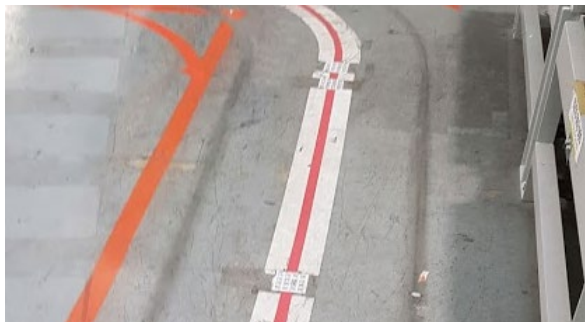
Figure 19: QR Codes on the Electrolux factory floor are read by the AGVs
