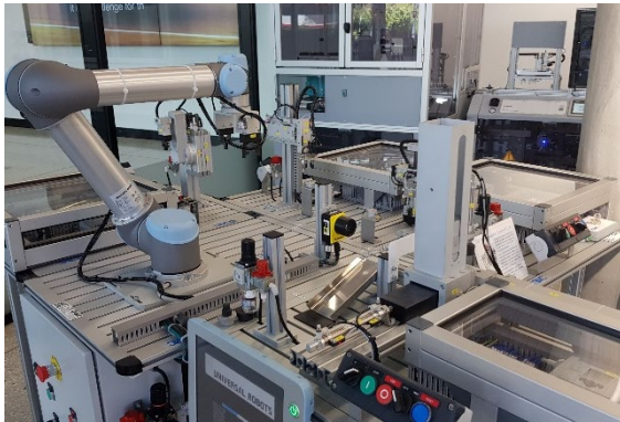
Figure 29: SMC Workstation with various sensors, mounted with a Cobot
