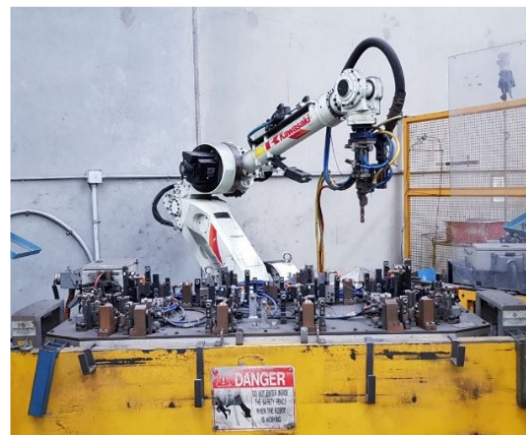
Figure 10: Kawasaki industrial robots spot welding at Multislide
