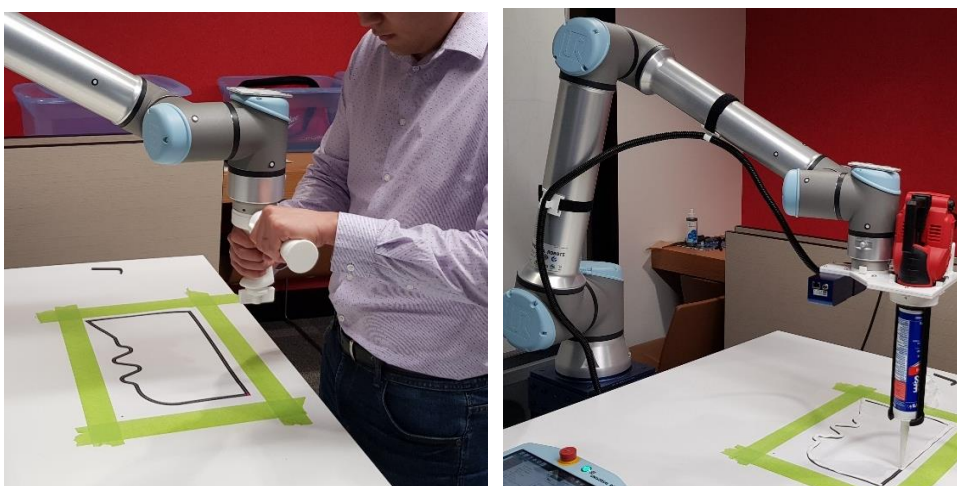
Figure 6: Teaching the glue path was followed by the cobot dispensing the glue
